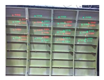
In the example below, white dots are showing where to measure and the colored ones have been measured and color represents the surface deviation from CAD nominal in 0.005" steps:
